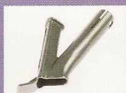
Speed welding nozzle 7 mm, triangle shaped for energy HT1600 127.833 Used with tubular nozzle 130.632
